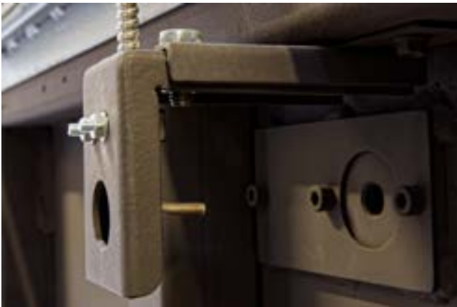
Detail view of the light guide for the receiver in curved design. The light guide head is located at some distance from the hole to the combustion chamber. (Image: ipf electronic)
