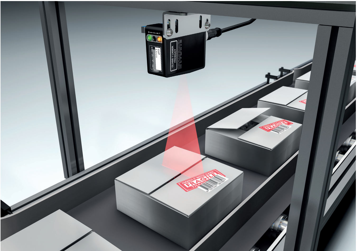
Gap detection on cardboard box flaps Image: ipf electronic
