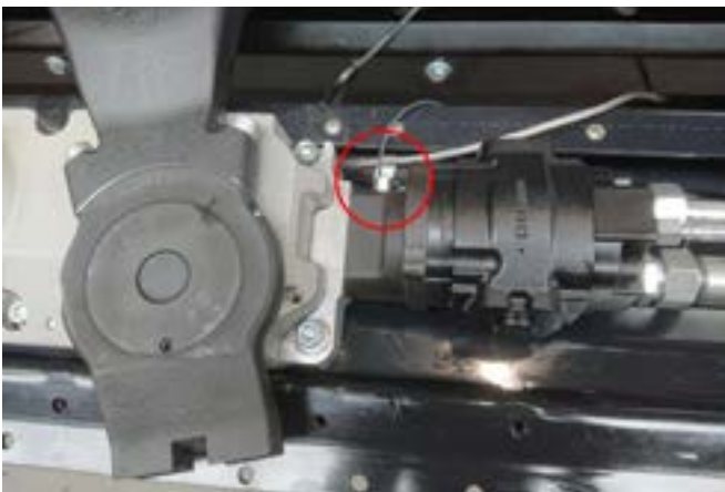
Detailed view of the gearbox flange: The hexagon on the IB08E337 inductive sensor ensures that the correct switching distance is maintained by means of the specified stop. (Image: Carl Geringhoff GmbH & Co. KG)
