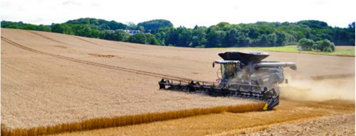
Special solution for large machines: ipf electronic developed a sensor for monitoring the speed of the blade drives in Geringhoff belt cutting units for combine harvesters. (Image: Carl Geringhoff GmbH & Co. KG)
