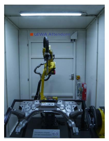
The cuboid LED light can be ideally integrated in the design concept of the robot welding cell and enables an optimum view of the entire work area.
