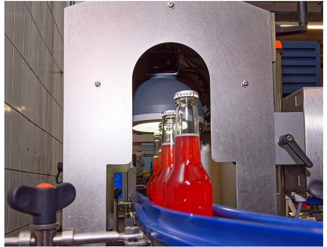
The OC539420 camera sensor detects crown corks of about six bottles per second vertically from above. The device is triggered by a customer's light barrier. Below the sensor, the dome light can be seen, which provides a diffused, shadow-free light. (Image: ipf electronic)
