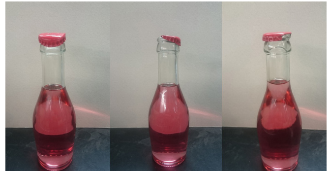
For preliminary tests provided bottles with defective crown corks. On the far right is a faulty closure, which is hardly recognizable neither from above nor from the side, depending on the position of the inspection system. (Images: ipf electronic)
