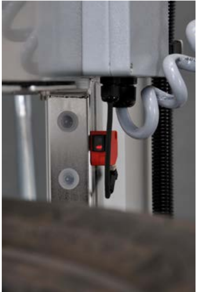
OR150175 retro reflective sensors for position inquiry of the lifting axis. Before clamping, the lifting axis is lowered until the upper edge of the green tire interrupts the light barrier. Then the inner grippers have also reached the correct height.
