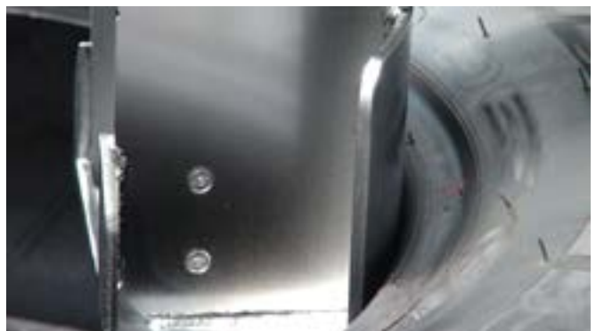
The gripper clamping process stops automatically, regardless of the tire's inner diameter, when both tire sidewalls have been reliably detected.
