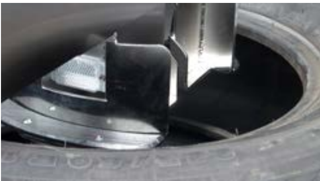
The switching distances of the two OT330570 optical diffuse reflection sensors in the grippers have been adapted to the slightly protruding tire supports. The reflector for the light barrier is also located in the movable gripper.
