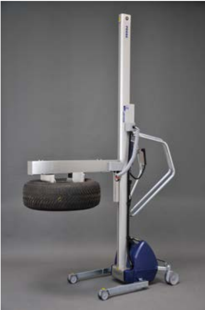
Semi-automated transport solution for green tires. The load pickup of the mobile lift consists of a lifting axis and a front fixed as well as a movable inner gripper. (All images: TransOrt GmbH)
