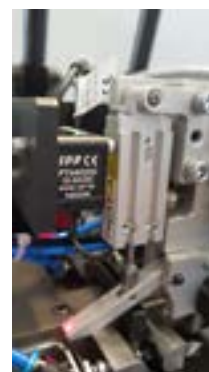
The analog outputs of the sensors provide a distance-proportional signal separately for each shift fork side, which is used for differential measurements.
