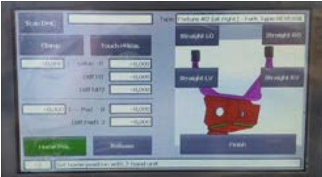
The worker in the Delhi plant is guided or instructed via software. It visualizes not only the deviations, but also the respective positions of the reversible lever for the individual straightening operations..
