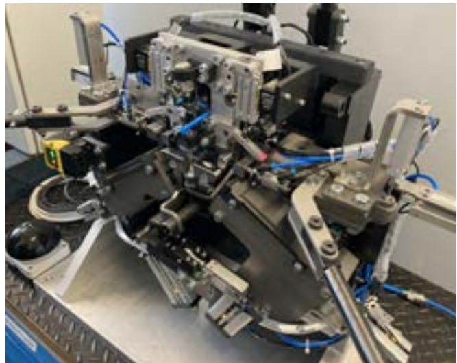
This special solution was developed by BEAS Technology for measuring and straightening shift forks. A central component is the area with the two sensors from ipf electronic for the measurements.
