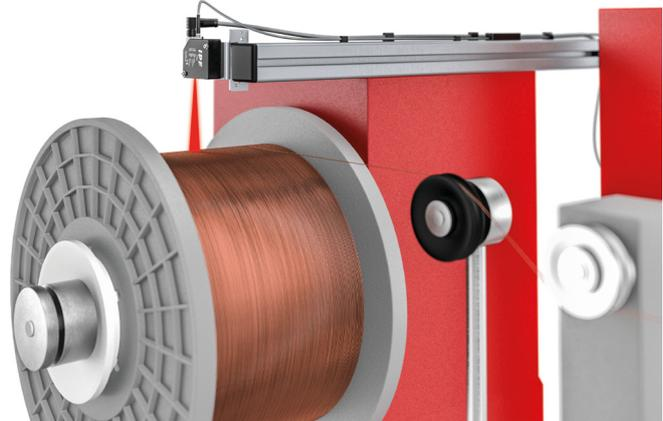
Even shiny, inhomogeneous surfaces such as a copper wire on a spool can be reliably detected with a **PT64** with laser line. In this application, the distance information is transmitted via the analog signal to a PLC in order to reduce the drawing speed of a machine or to stop the machine depending on the respective sensor signal.
