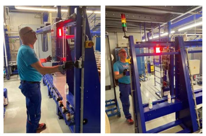
A total of three cameras are installed in the plant. The figure shows the area of the infeed. There, the substrates are marked with a 2D code and immediately verified via a camera system. (Prinz Optics GmbH)
