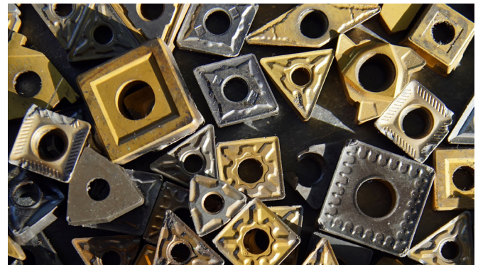
During machining, inserts for metalworking are subjected to high mechanical stresses, as these used tools show. The "recipe" for the cutting materials is therefore crucial for long tool life, apart from the material being machined. (Image: Adobe Stock)
