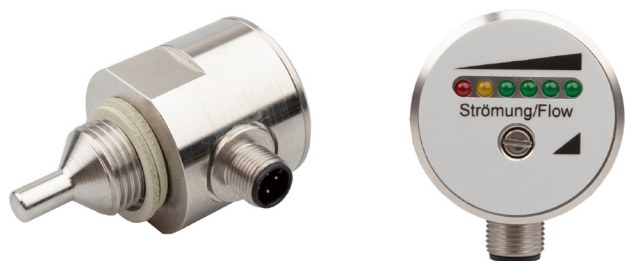
A glance at the LED indicators is enough to determine whether there is sufficient flow or not. The robust SS410124 from ipf electronic is designed for media temperatures up to +80°C and is pressure-resistant up to 100bar. Housing and sensor are made of stainless steel 1.4571 and have protection class IP67. The flow monitor operates according to the calorimetric principle and is absolutely wear-free.
