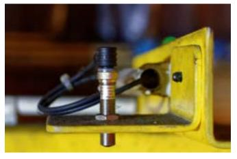
The transmitter unit of the high-performance light barrier. The selected aperture angles allow the transmitters and receivers to be easily aligned with each other, even at ranges of up to 60 meters.
