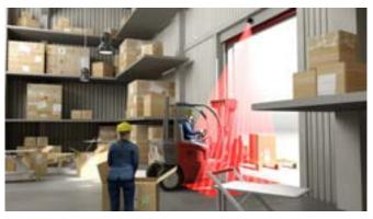
If a vehicle stops in the door area, the presence check of the sensor ensures that the door remains open until the vehicle leaves the detection range of the **RO710900**. Vehicles that merely drive past the gate or persons moving within the detection range of the radar sensor are reliably blanked out.
