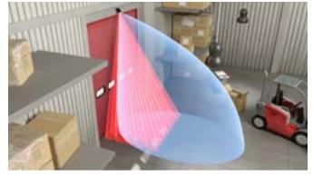
The sensors from ipf electronic enable reliable motion control and, due to the active infrared technology, presence control of objects at the same time. The coverage area of the IR field can also be adjusted individually via a remote control at a later date. All images ipf electronic.
