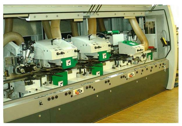
Different frequencies have to be evaluated for the spindle drives of the different drives: Up to 70Hz in the case of standard machines, up to 300Hz in the case of high speed aggregates and up to 800Hz in the case of high speed spindles.
