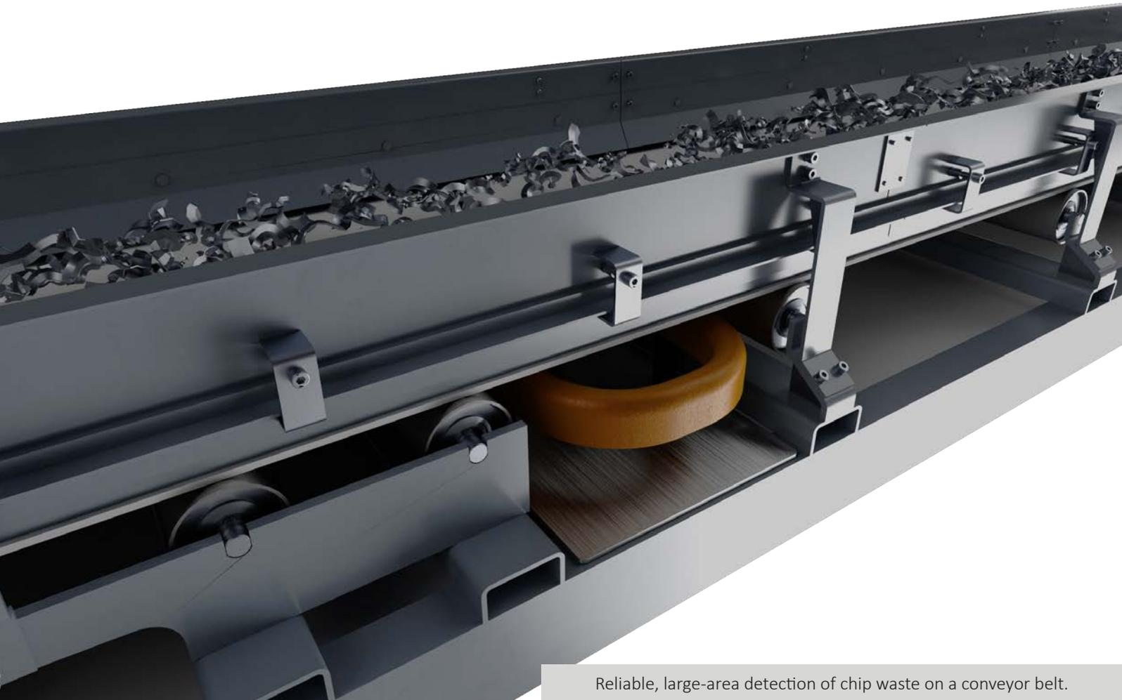
Reliable, large-area detection of chip waste on a conveyor belt.
