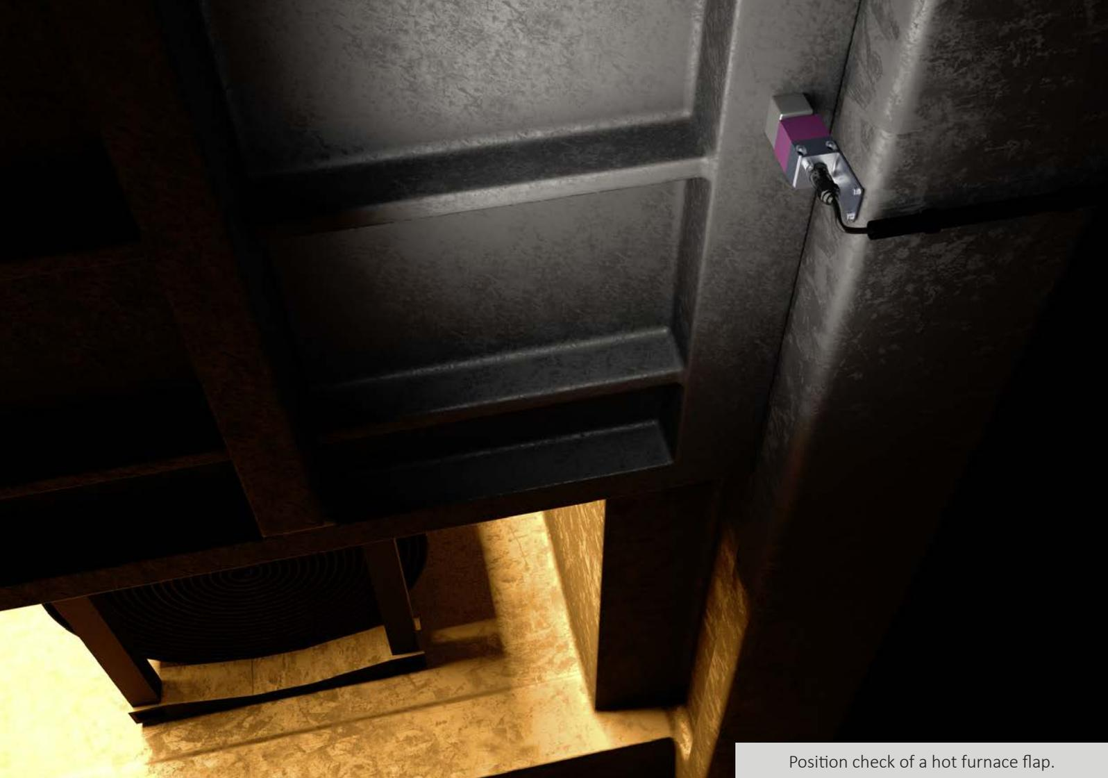
Position check of a hot furnace flap.
