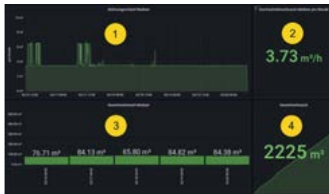
The visualization software was used to create a wide variety of flow diagrams over the course of the project. It was also possible to select individual detailed views with an enlarged display and higher measured value resolution. This visualization shows the flow curve (1) and the average flow curve (2) in m³/h, the daily consumption of compressed air (3) in m³ and the total consumption (4). (Image: DTS GmbH)
