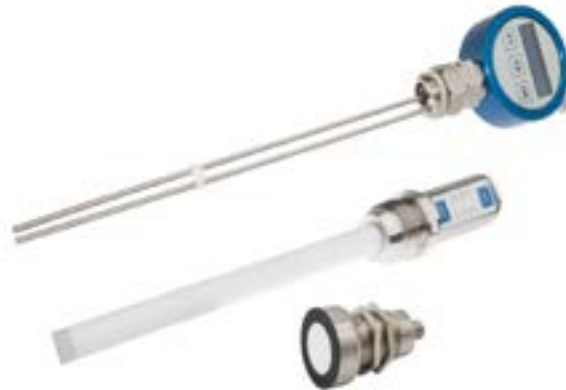
Various solutions from ipf electronic for level measurement: FM -series sensor with parallel rod and integrated switching output for immediate use without media adjustment (top), an FK -series device with measuring probe for media temperatures up to +100°C (middle) and an ultrasonic sensor from the UT -series with long range for non-contact level measurements (bottom).
