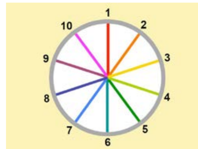
Certain knowledge from the theory of color can be helpful. The figure shows a color wheel in which the complementary colors are directly opposite one another. 1 red, 2 orange, 3 yellow, 4 yellow-green, 5 green, 6 blue-green, 7 blue, 8 blue-violet, 9 violet, 10 magenta. (Figure: ipf electronic gmbh)
