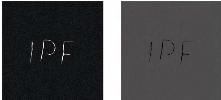
Scratches on acrylic glass. Left: With dark-field transmitted light illumination, the artifacts stand out as bright areas. Right: Bright-field transmitted light illumination.
