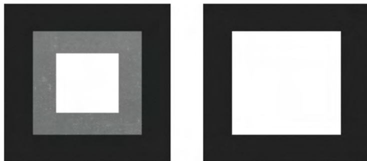
Deep hole. Diffuse transmitted light (entocentric lens) (left). Telecentric transmitted light (telecentric lens) (right).
