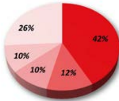
Savings potential in compressed air generation: 42%: Identification and elimination of leaks 12%: Design of the pneumatic system including a multi-pressure line network 10%: Heat recovery. 10%: Compressors with variable motor speed 26%: other measures
