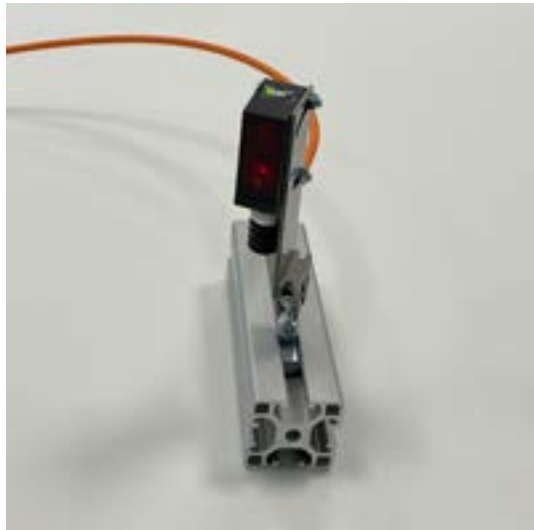
ON450522 auto-reflective sensors with outstanding features: switching frequency 2kHz, response time \leq 0.25\text{ms} and range up to 1,000mm.
