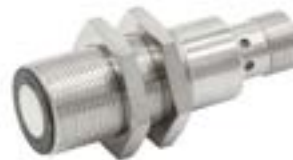
Ultrasonic diffuse-reflection sensors such as the UT189520 can be easily switched to a retro-reflective sensor via IO-Link and can therefore be set to a background instead of an object in order to reliably detect transparent objects with irregular, round or angled surfaces, for example.
