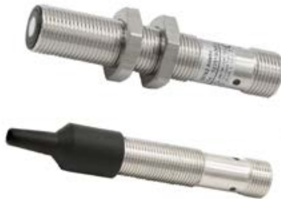
Fig. 31: The sonic nozzle on the sensor head of the UT129021 focuses the ultrasound so that levels in containers with very small openings can be scanned.
