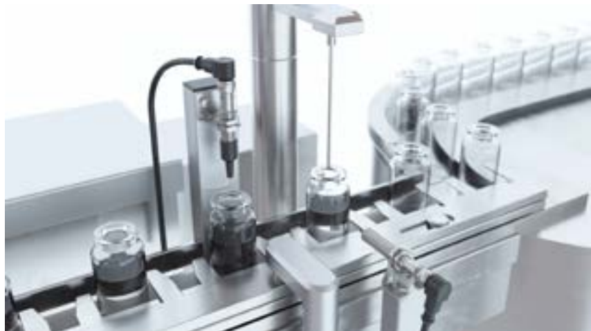
Fig. 32: The UT12 series ultrasonic sensors in the automated dosing unit: A sensor with switching output is used to check presence. The device behind the dosing unit checks the fill levels from above through the small bottle openings.
