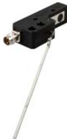
Fig. 26: Level sensor F1520172 for a vibratory feeder. The pendulum is made of stainless steel. The thickening in the upper area can also be seen, which is used for interrogation with the inductive proximity switch integrated in the holder.
