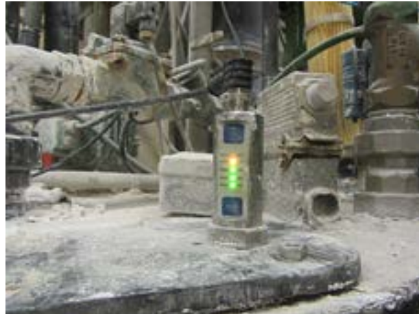
Fig. 33: Housing and connection of the capacitive level sensor are made of stainless steel. The limescale deposits are also clearly visible on the container of the preparation unit.
