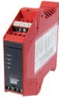
Fig. 8: In addition to level or limit detection of electrically conductive media, also in plastic containers, the FV56 field devices can be used in conjunction with the probes for overflow protection of containers with non-flammable, water-polluting liquids.
