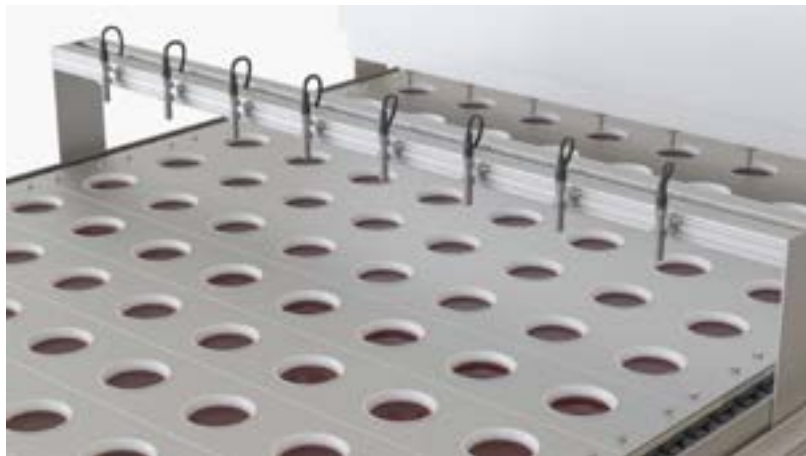
Fig. 19: Filling level control with several IO-Link ultrasonic sensors at a filling station.
