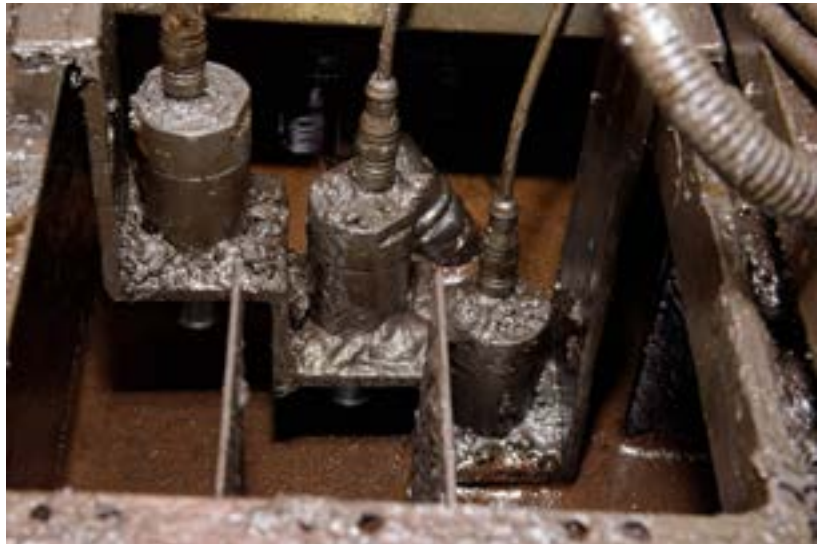
Fig. 6: FK92 series sensors in a reservoir for permanent lubrication of punching tools.
