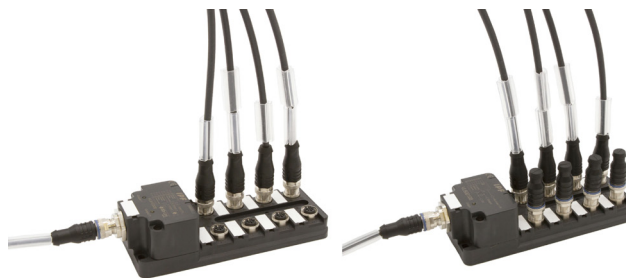
Simulation plugs for vacant slots in AND operations, as in a logic distributor without IO-Link interface (right), are no longer required with the IO-Link logic modules (left). Among other things, this leads to further material and cost savings.
