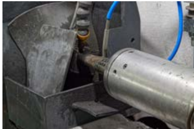
Using the ultrasonic head and a soldered-on negative die, the appropriate shape is carved into a stone using high vibrations and boron carbide.
