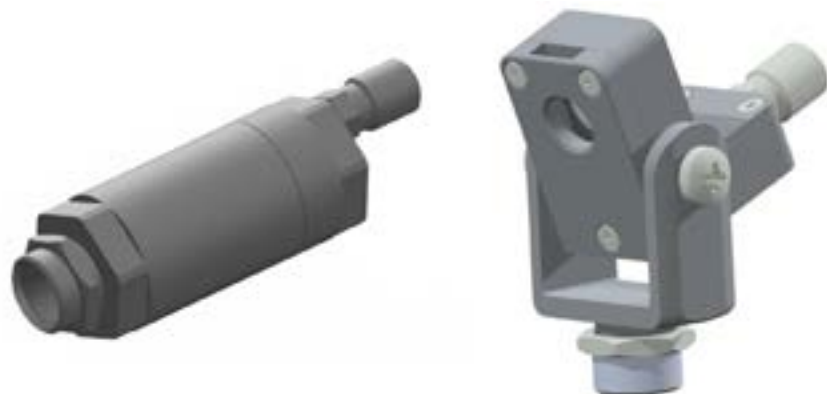
Fig. 5: To prevent contamination of the optics, either standard air purge attachments (left) or air purge attachments with lateral air outlet can be used. The laminar air purge attachments (right) prevent the object from cooling down at small measuring distances.
