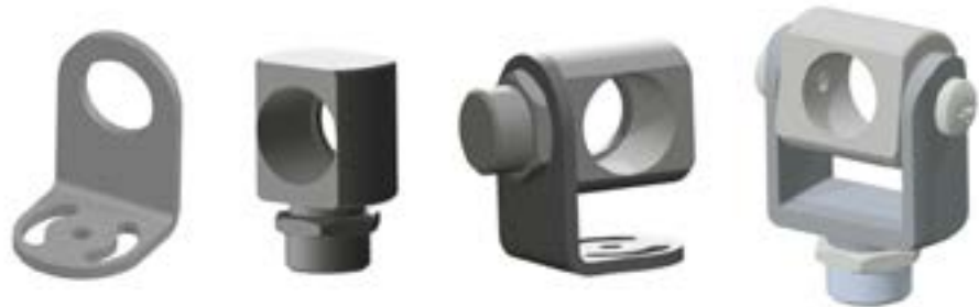
Fig. 4: A range of accessories is available for mounting the measuring heads for the two-part systems. Left: a mounting bracket and next to it a mounting bolt (each adjustable in one axis) as well as the combination of both solutions (adjustable in two axes). Far right: a mounting fork that can also be adjusted in two axes.
