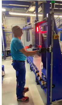
A total of three cameras are installed in the system. The illustration shows the infeed area. Here, the substrates are marked with a 2D code and verified directly via a camera system. (Prinz Optics GmbH)
