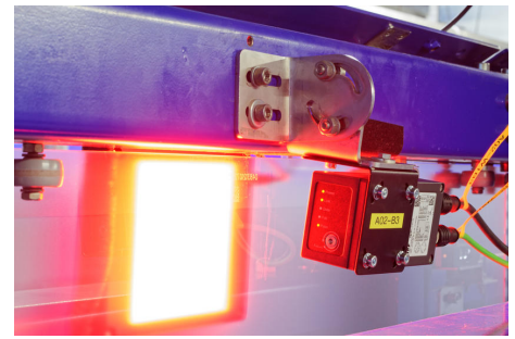
One of the cameras in use. Thanks to transmitted light as the lighting technology, interfering reflections or the quality of the labeling are no longer relevant for reliable recognition. (Image: ipf electronic gmbh)
