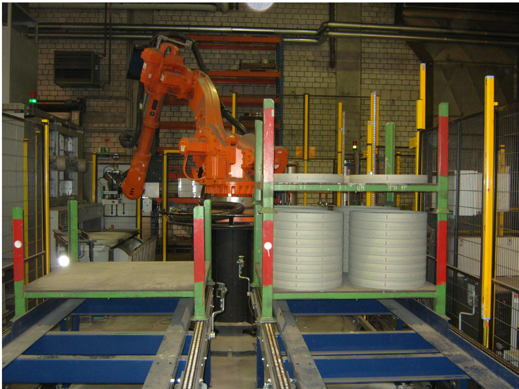
Automated loading of an oven belt Image: ipf electronic
