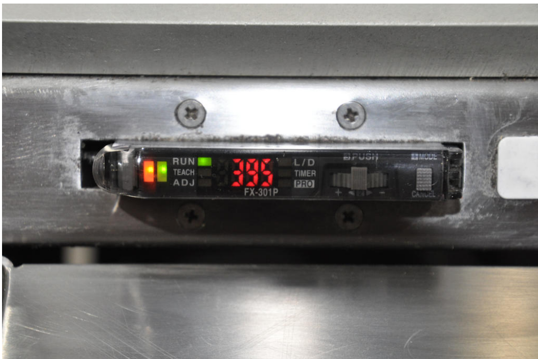
Detailed view of the amplifier. The displayed value shows the signal strength of the light barrier when the light signal is interrupted.
