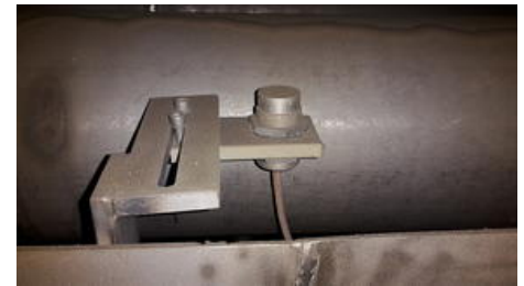
The inductive sensors have an active surface made of stainless steel and are therefore very robust (protection class IP68) and designed for ambient temperatures up to +70° C.
