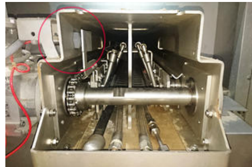
The two inductive sensors IB1201K0 for linear measurement and inquiry of the direction of rotation are mounted in front of a coding disk on the driveshaft (left) of the chain drive. (Image: IBS Paper Performance Group)
