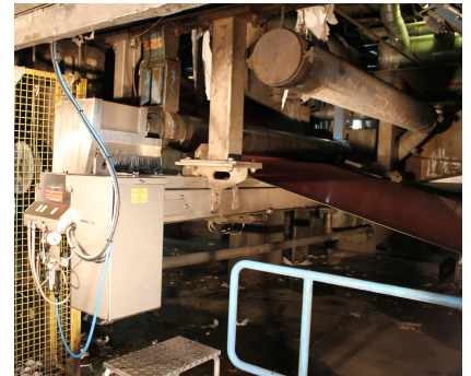
View of a paper machine. Part of the machine clothing supported by rolls can be seen on the right. (Image: IBS Paper Performance Group)
