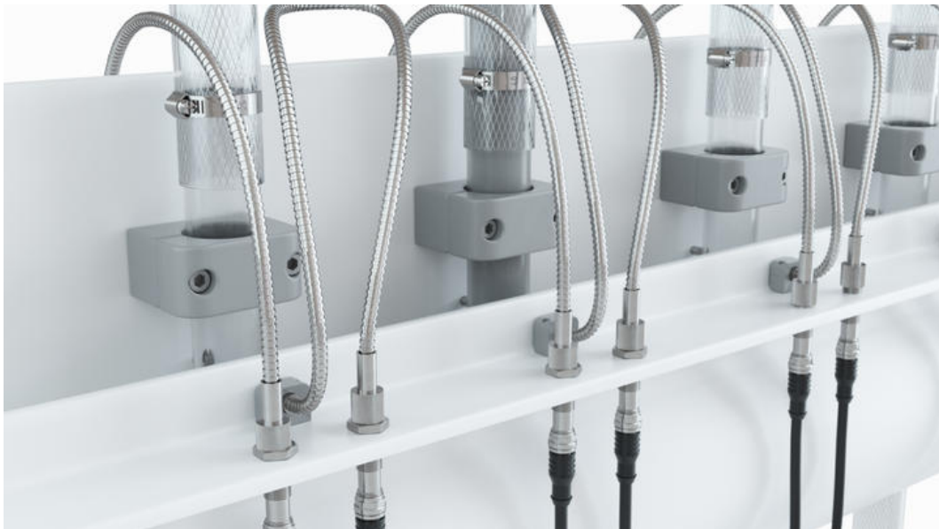
If the infrared light beam of the light barrier, consisting of an optical transmitter OS126020 and an optical receiver OE126020is interrupted due to clouding of the coolant in one of the glass tubes (second tube from the left), the relevant evaluation channel of the connection unit generates a switching signal.
