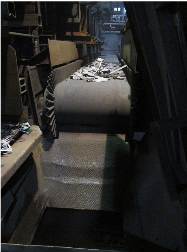
The conveyor belt in the area of the discharge chute (here from two different perspectives). The pictures clearly show that very rough operating conditions prevail here.
