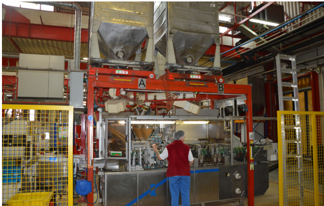
The operating staff at the filling plant receives a message as soon as a raw material container above the filling station is empty. Then, the plant is switched to the second, full container and a request is sent for a forklift truck driver to replace the empty container. (all images: ipf electronic)
