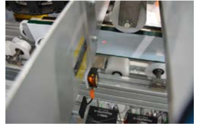
Lechenauer opted for the PT430470 laser light scanner, which generates a very precise laser spot for a trigger signal.
