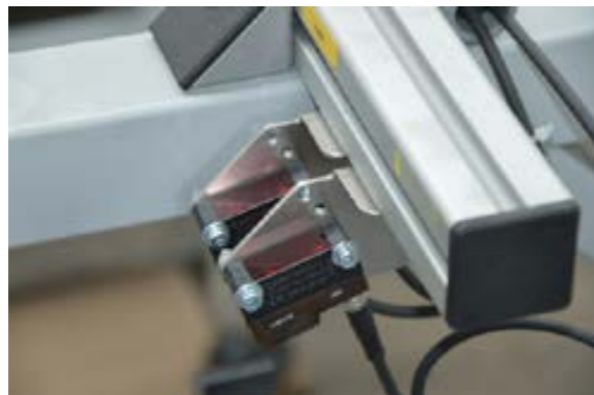
The non-contact optical sensors of the OT43 series have a maximum switching distance of 600mm. The devices in IP67 have been mounted inside the plant so that they are relatively insensitive to contamination.
