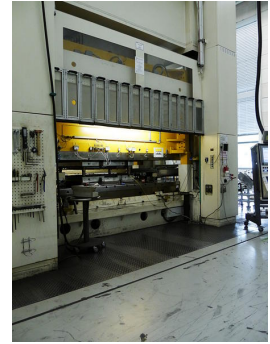
Press for the production of cylinder-head gaskets. Production takes place from a running steel coil, with the individual layers of the multilayer steel gaskets (MLS gaskets) being manufactured in progressive dies that combine several work steps.
