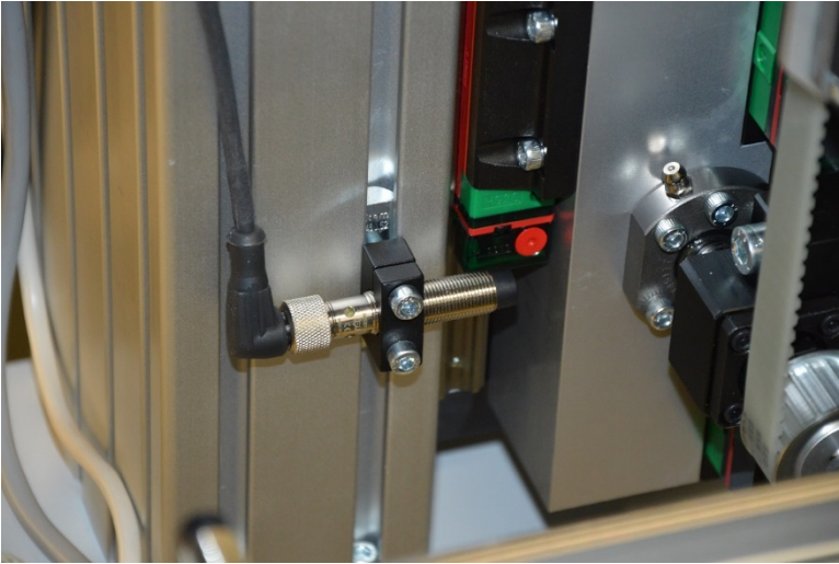
Image caption ipf_app_MD_Automation_04.jpg: A feature of the IM120120 is the encapsulated electronics in a robust metal housing (protection class IP67) to protect it against shocks.
