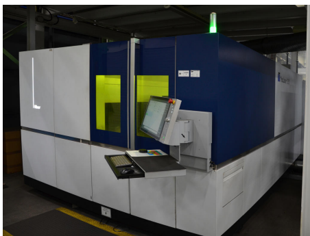
In the course of investing in new laser cutting systems, e.g. a TruLaser 5030 fiber from Trumpf, Kettenwulf is taking a closer look at their consumption.
