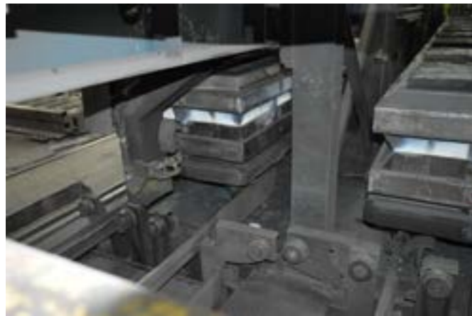
At this position within the station, the sensors must detect the presence of a casting container.
