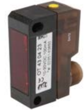
Not only robust, but also reliable under adverse ambient conditions: The OT430423 with protection class IP67 is suitable for application temperature ranges from -25°C to +65°C and reaches a sensing range of 30 to 500mm.
