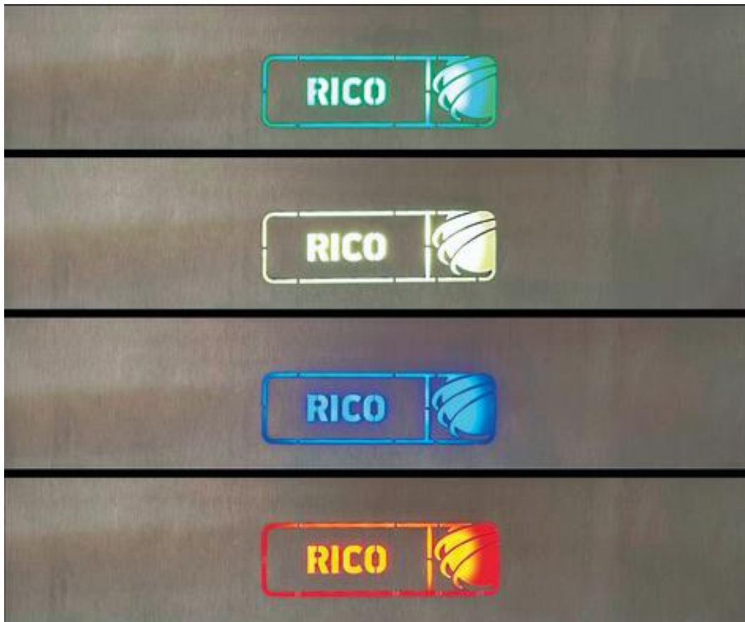
Four handling statuses are displayed via the logo: Automatic mode (green), setup mode (yellow), connection to a network (blue) and interference (red). (Image: ipf electronic gmbh)
