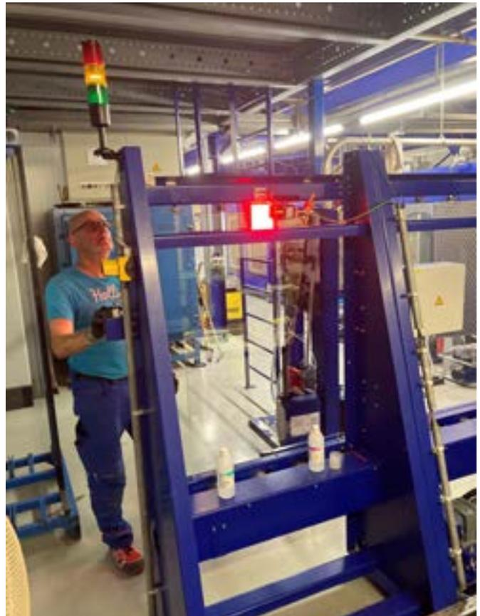
A total of three cameras are installed in the plant. The figure shows the area of the infeed. There, the substrates are marked with a 2D code and immediately verified via a camera system. (Prinz Optics GmbH)
