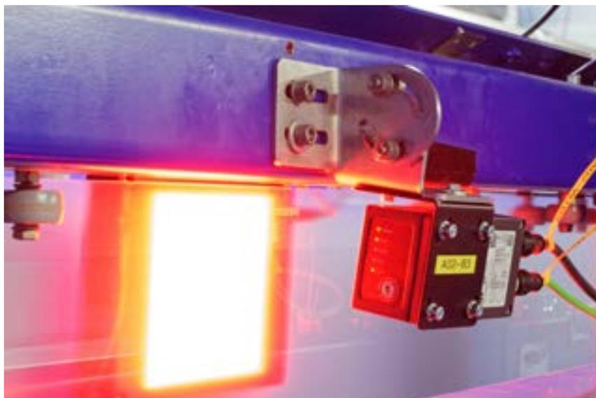
Layer tracking means that the marking is always reliably recorded and the code identified.(Image: ipf electronic gmbh)
