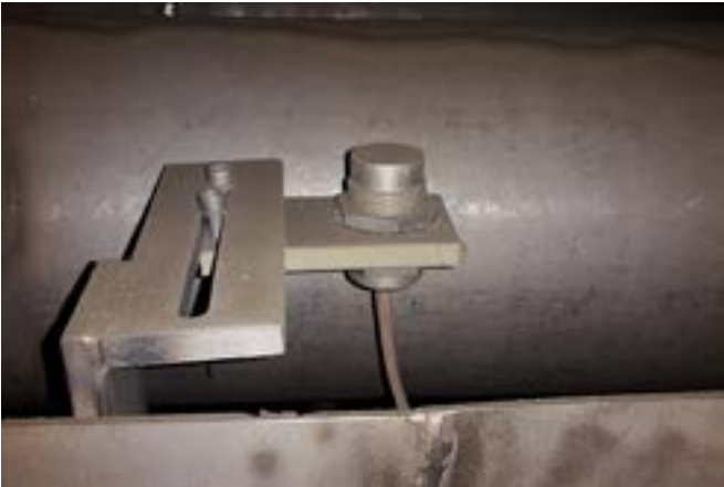
The inductive sensors have an active surface made of stainless steel, are therefore very robust (protection class IP68) and made for ambient temperatures of up to +70°C.
