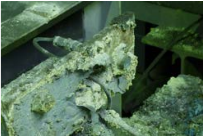
The acid-containing pickling extremely damages the laser light barriers in the buffer zones, as can be seen clearly, but the sensors installed just above the roller conveyors work reliably.
