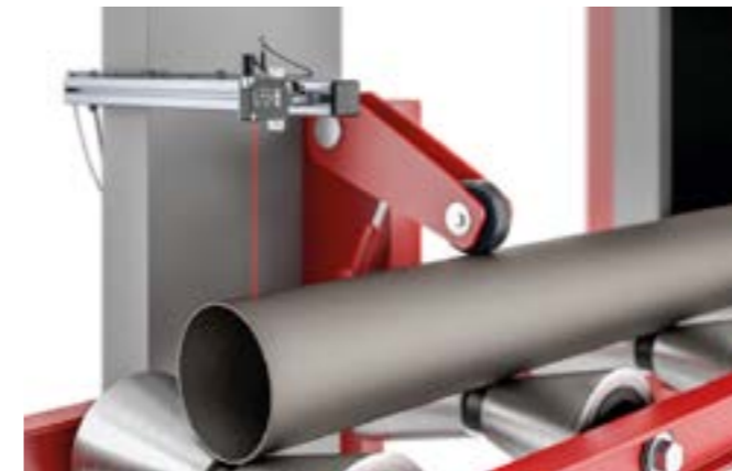
The drag pointer function can be used to check the ovality of pipes with a specific diameter.
