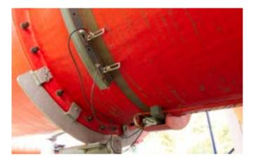
View under the cover at the end of the tube. Two systems were installed here, with transmitters (top) and receivers (bottom) of a light barrier mounted alternately on each side of the slide.
