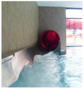
The exit of the slide opens into the indoor pool of the four-season pool. For safety reasons, the water slide is only released when both lower light barriers switch. The traffic light in the indoor pool then changes to green with a time delay of 4 seconds.
