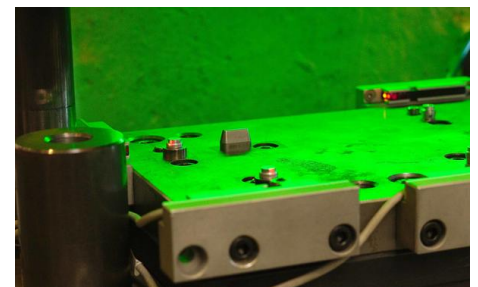
The light color of the signal light changes to "green" as soon as the light receives the logic operation AND signals from the optical sensors. All bolts are then present in the tool and can be pressed into the component.
