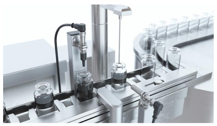
Ultrasonic sensors of the **UT12** series in an automated dosing system: The device behind the dosing unit monitors the filling levels from above through the small bottle openings. Another sensor with switching output is used to perform the presence check. (All images: ipf electronic)
