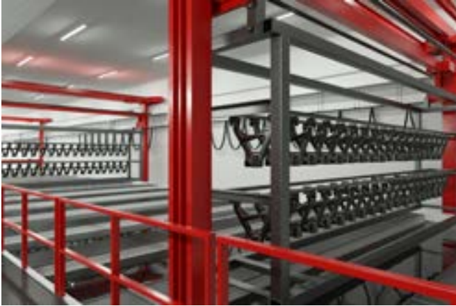
The entire CDC process requires 12 individual process steps and consists of multiple large baths arranged one after another. (All images: ipf electronic gmbh)
