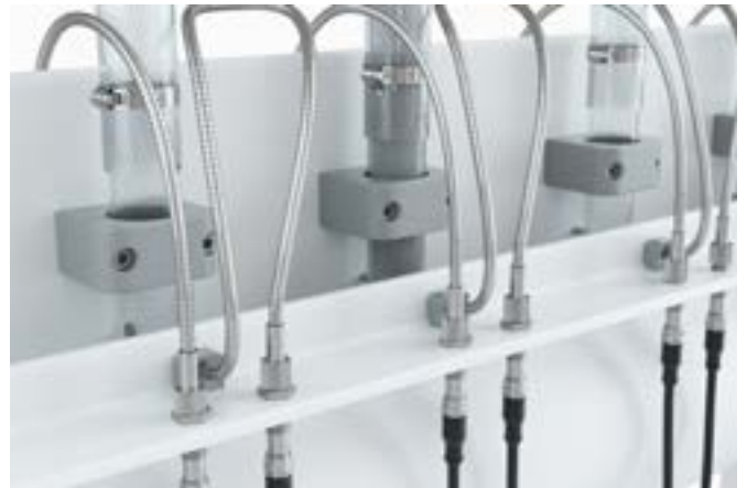
If the infrared light beam of the light barrier, which consists of an OS126020 optical transmitter and an OE126020 optical receiver, is interrupted due to the coolant in a glass tube becoming cloudy (second tube from the left), the relevant evaluation channel of the connection unit generates a switching signal.
