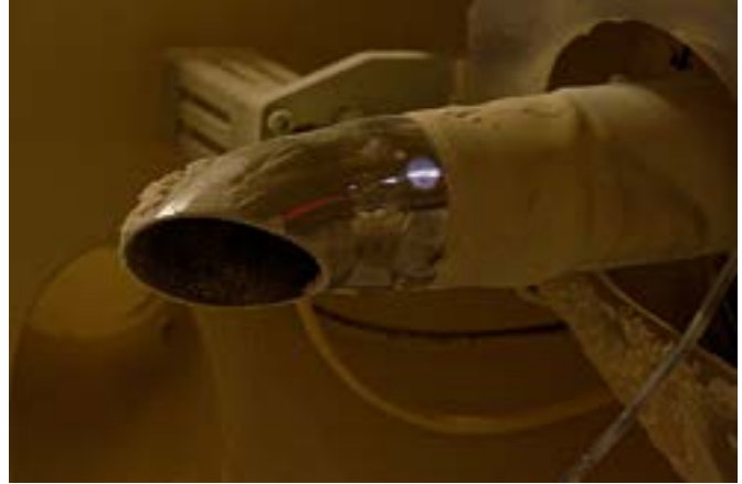
ipf electronic_Farbsensor_Weizen_Roggen-Mühle_002.jpg: To achieve the highest possible illuminance at the required working distance of 280mm, a so-called XXL lens in the M34 design was used instead of a standard zoom lens.
