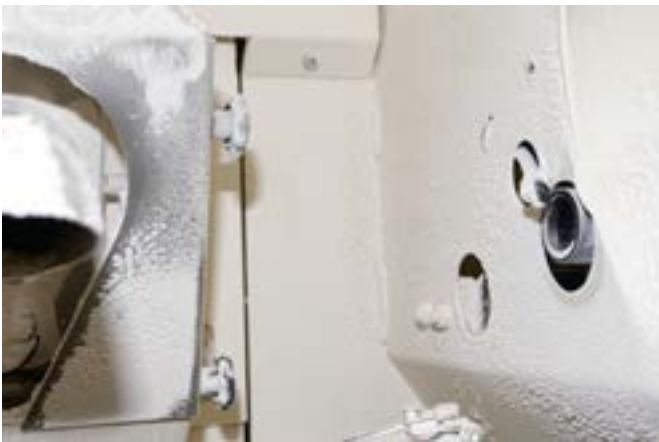
ipf electronic_Farbsensor_Weizen_Roggen-Mühle_003.jpg: Front side of the OF650180 color sensor with a blow-off device to remove flour dust from the optics.
