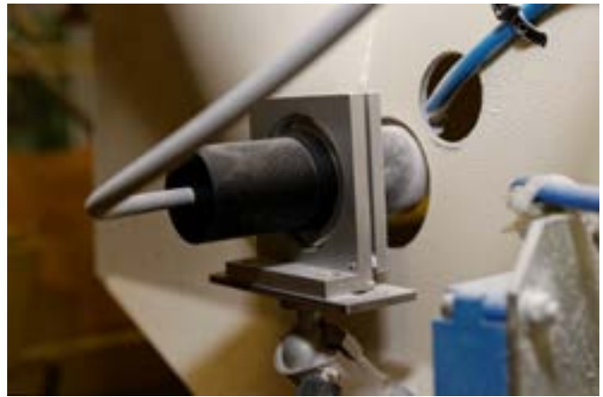
ipf electronic_Farbsensor_Weizen_Roggen-Mühle_004.jpg: Rear view of the application: An opening was created on a side wall of the automated filling line for the color sensor.
