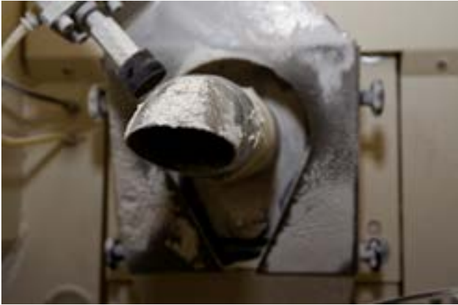
ipf electronic_Farbsensor_Weizen_Roggen-Mühle_001.jpg: The paper bags are automatically filled through a spout on which flour is deposited. These varying flour deposits posed a particular challenge during the development of the sensor solution.
