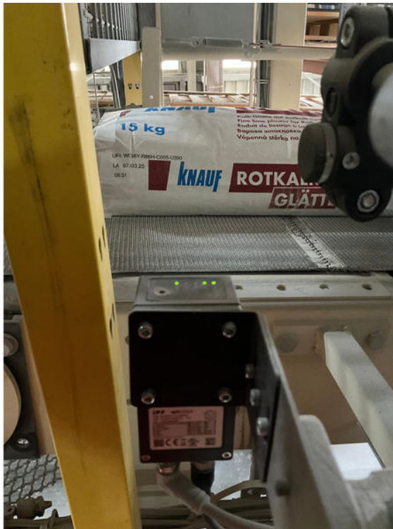
An average of 1,500 sacks per hour per production line are certified by the camera sensors (one device in the foreground). Knauf Gips KG, Lauterhofen plant)
