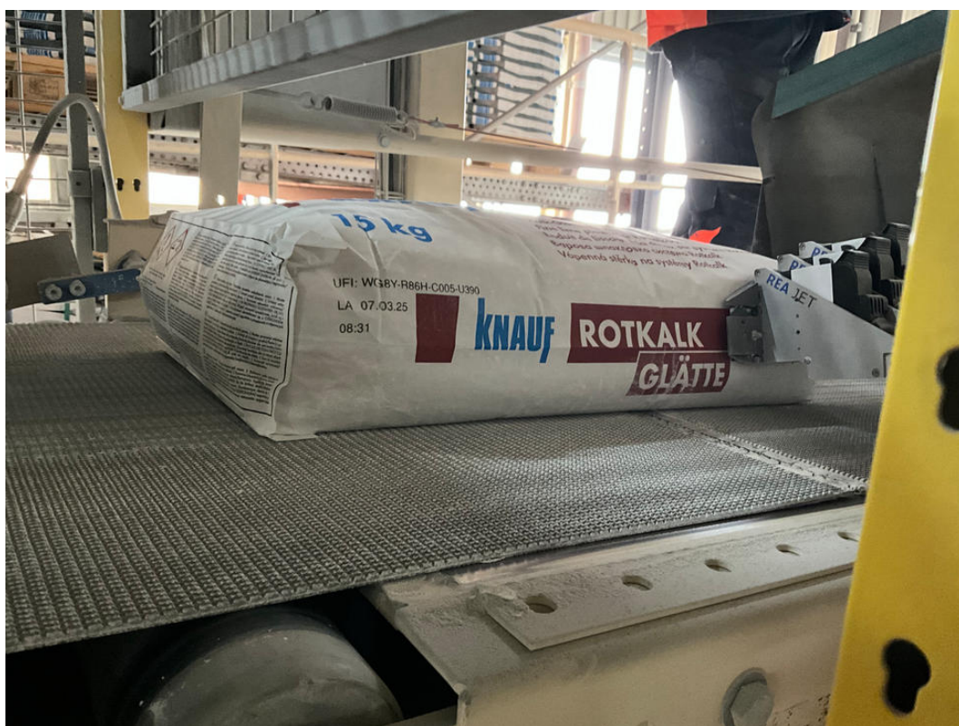
The three-line marking on the packaging includes the UFI code, the abbreviation of the Lauterhofen plant (LA), the production date and the time. (Image: Knauf Gips KG, Lauterhofen plant)
