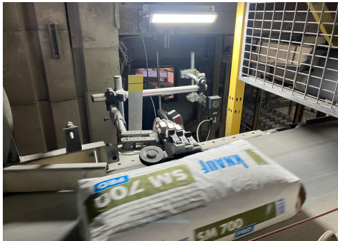
A compact camera from the OC53 directly behind the printer seamlessly checks the quality of the labeling on the packaging with finished products. (Pictures: ipf electronic)
