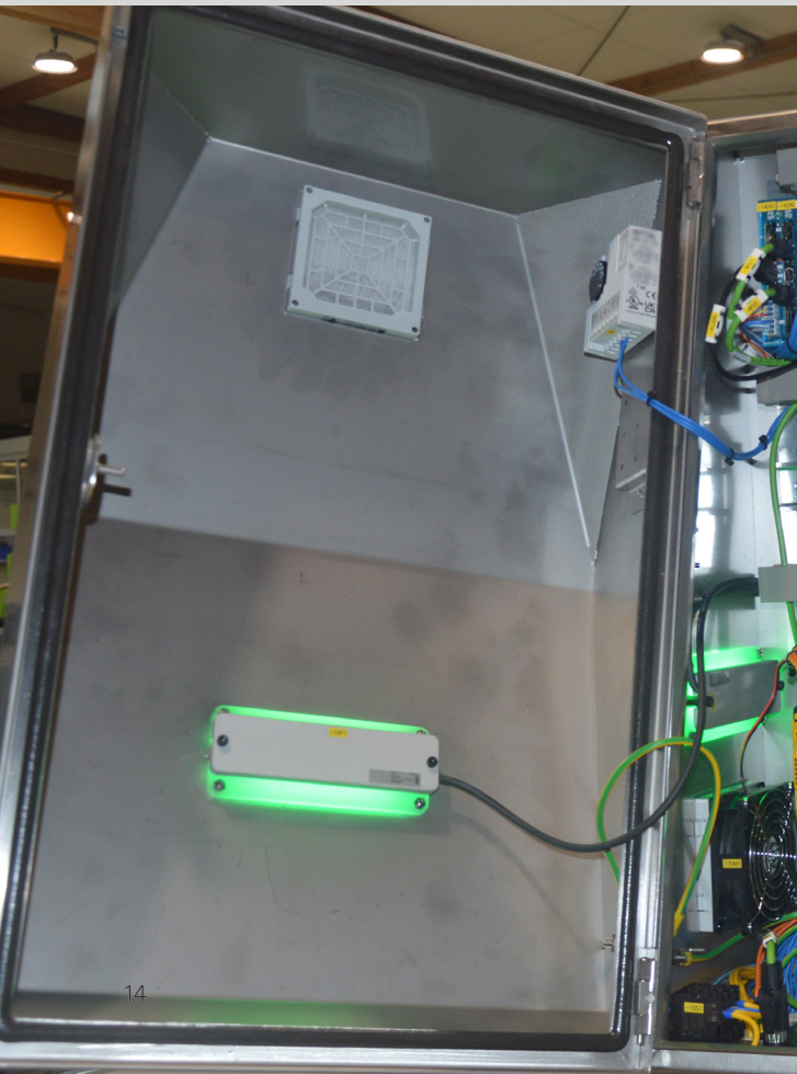
Company logo as status display on demolding handling systems for injection molding machines
