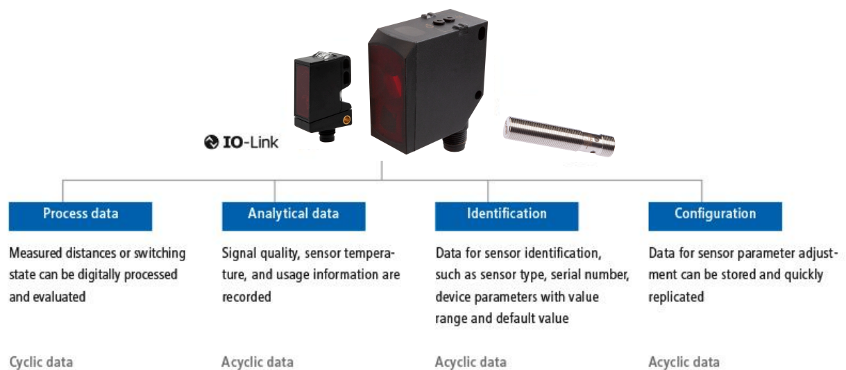
Figure 2 Different IO Link data streams
