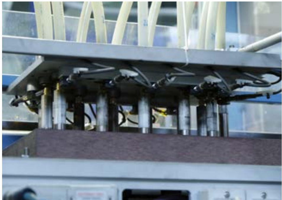
Equipping device for brass bushes. The inductive sensors with IO-Link interface inform the higher-level PLC if they no longer have a sufficient functional reserve.
