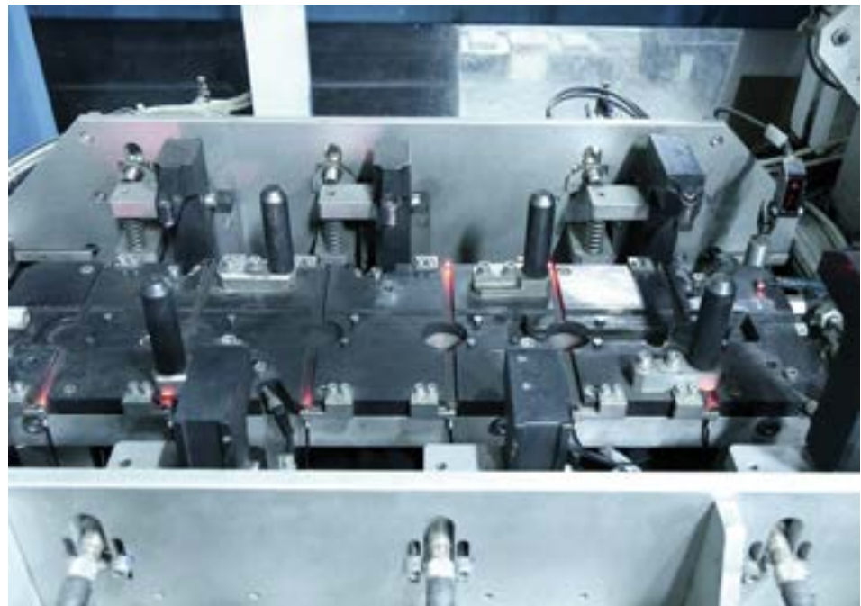
By replacing conventional sensors with IO-Link devices, spare-parts stock could be reduced and, thus, storage costs minimized.
