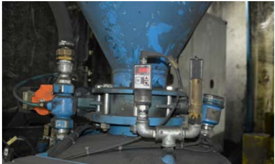
Fig. 2: Pressure sensors of the series DW34 , DW 35 and DW36 are suitable for various pressure measurements of gases and liquids. Here is a pressure sensor of the DW35 series for monitoring a transport pipe filled with compressed air for dust, which is produced in nodular cast iron and is discharged into a silo.
