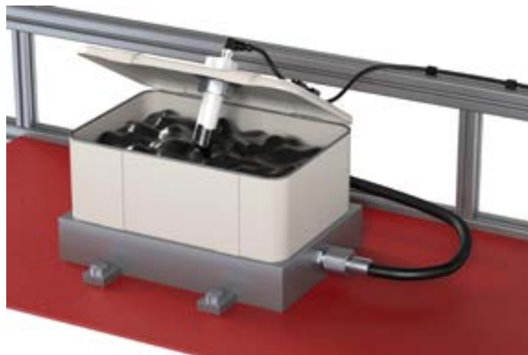
Fig. 14: Capacitive sensor FK920420 for monitoring the level in a container, which contains graphite paste for permanent lubrication of a tool.
