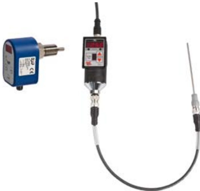
Fig. 5: One-piece and two-piece temperature sensor for PT100 (from left). The two-part version with separate evaluation electronics has wear-free transistor switching outputs (1A per channel).
