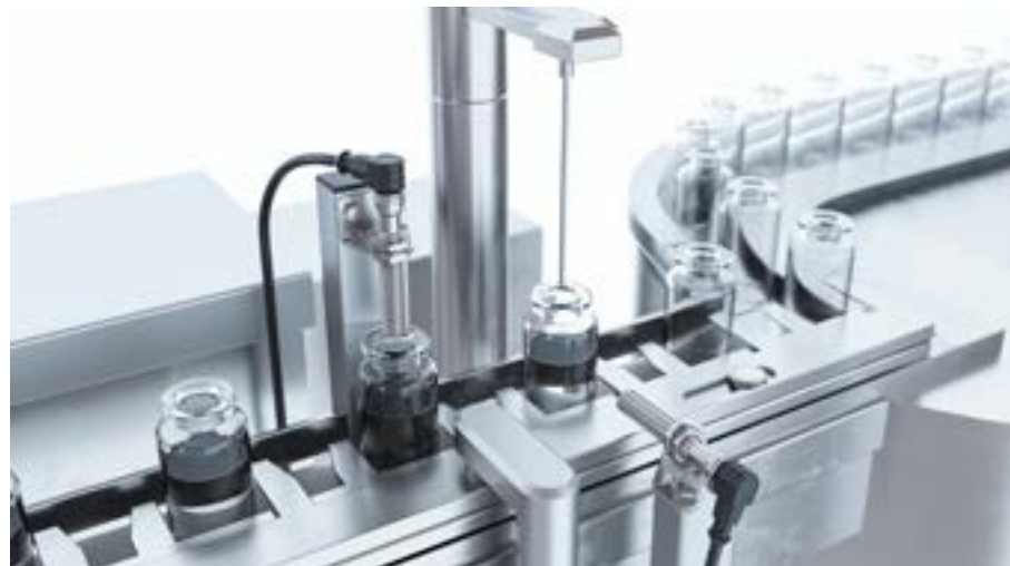
Fig. 18: Ultrasonic sensors of the UT12 series in an automated dosing system of a chemical company. The sensor behind the dosing unit (left) controls the filling levels from above by the small bottle openings. A further sensor with switching output is used for presence monitoring.
