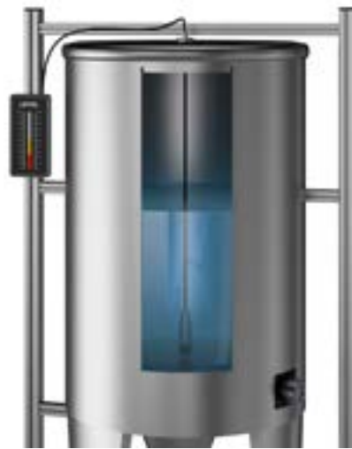
Fig. 17: ipf's hydrostatic pressure sensors (here a "hanging installation" in a container) have degree of protection IP68 and are suitable for media temperatures from -20°C to +70°C.
