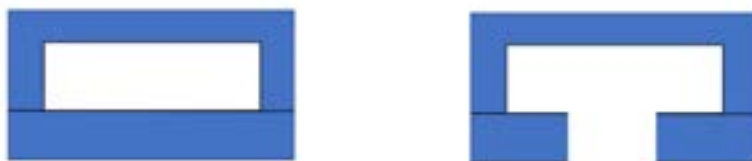
Fig. 1: Absolute pressure (left): The measurement is performed against a closed room, usually a vacuum). Relative pressure (right): The measurement is performed against an ambient pressure.
